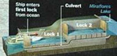
Water from Miraflores Lake enters first lock through culvert system, elevating ship to level of second lock
